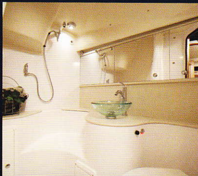
The large head is made from a single piece fiberglass molded part that creates a sculptured appearance and is easy to clean
