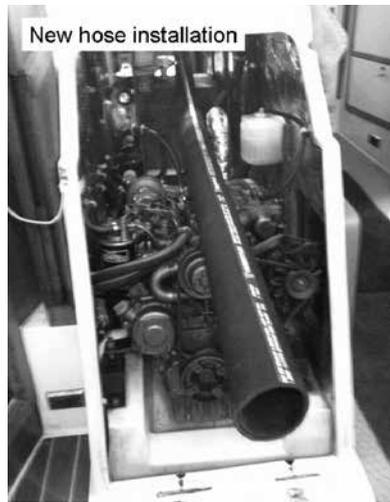
the exhaust opening in the transom during the replacement. Photo 7 shows the new hose during installation.
