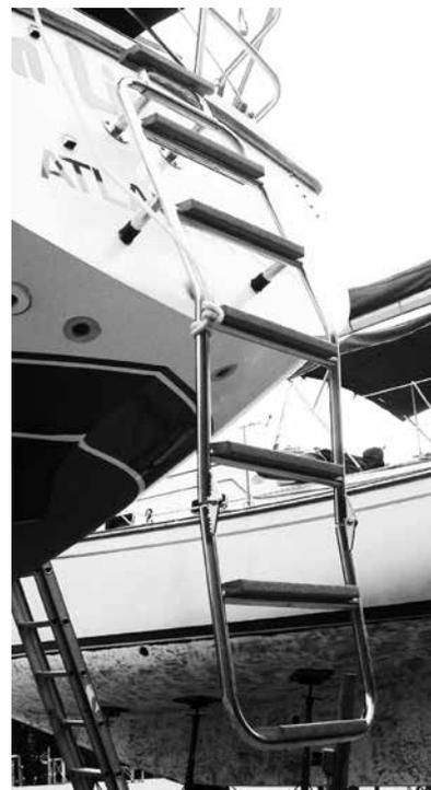
Design for new bi-folding ladder that would extend 3 rungs below the waterline.
