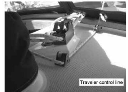
port and starboard orientation. I had to rethread the control line on the traveler so it would come over the top rather than through it. Photos 8 and 9 show the new arrangement.
