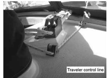
port and starboard orientation. I had to rethread the control line on the traveler so it would come over the top rather than through it. Photos 8 and 9 show the new arrangement.
