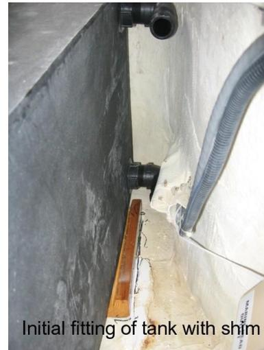
With the tank in-place, pull a hose from tank space to the head and attach the hose to the toilet fitting. Allowing the hose to make a wide turn around the outboard end of the tank (see picture,) mark the hose for the top fitting on the tank and cut with the hack saw.
