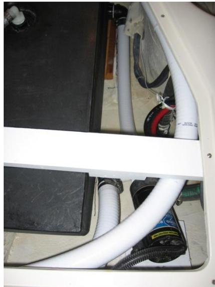
once again removed, attach the short lower fitting on the tank. Double you won’t be able to do this in-place. the space so that lower fitting is entrance and rotate the tank partly to fitting above edge of entrance. Now, fitting on tank to the macerator pump may leave the clamps loose for now. upper the upper fitting on tank with tank up to vertical, lower tank into rotate to starboard as the tank slides tank to marks on the hull made in-place with all but the deck hose
