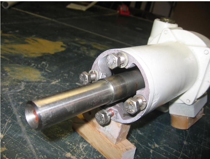
four bolts, and the unit can be removed from the V-berth. Note that the mounting ring is held in-place by 4 more bolts accessed only from inside. These do not need to be removed. After the four mounting bolts are removed inside the anchor locker, from the V-berth you can slide the unit towards starboard and drop it towards you. It's really quite easy.
