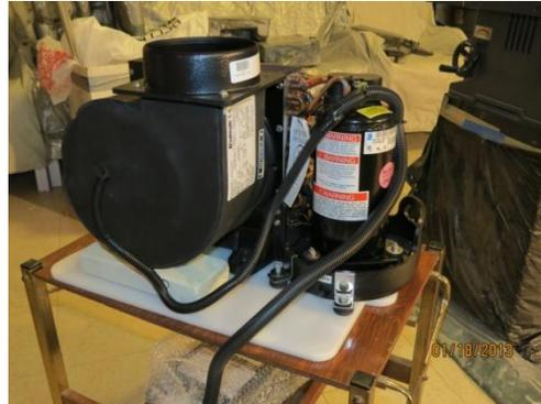
Since the port locker is not originally part of the space intended to be cooled, it is necessary to enclose the unit to prevent incursion of outside air. Failing to do so will allow unconditioned air and humidity to be drawn into the return air flow. This will greatly impact the efficiency of the unit. The design and construction of the cover will be discussed later.
