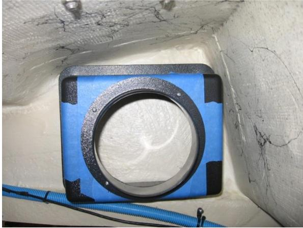
Using a pencil, reach inside the box while in-place and scribed the corners. Using a straight edge, scribe a line diagonally from each corner so the lines cross in the middle. Then, where the lines cross, drill a hole through the bulkhead. This hole will help to locate the grill on the galley side.
