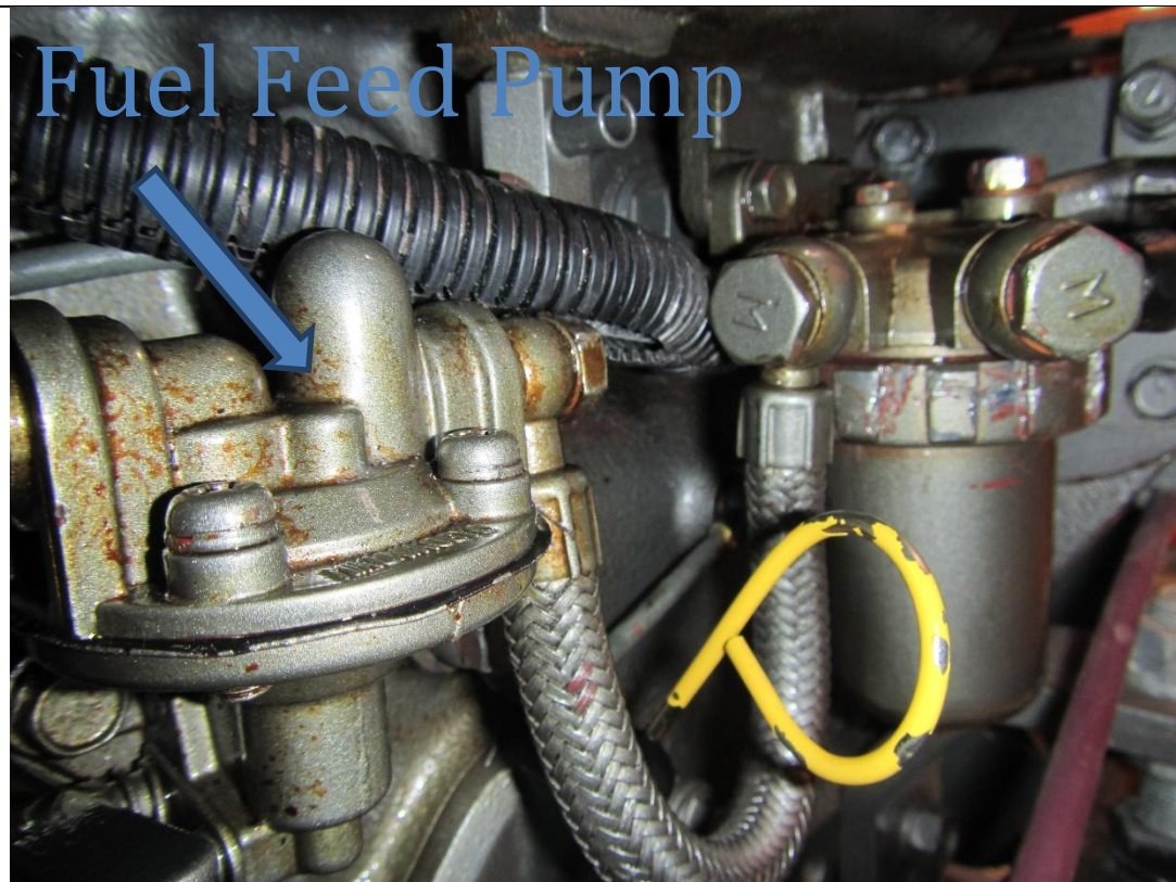
Figure 1 Fuel Feed Pump
