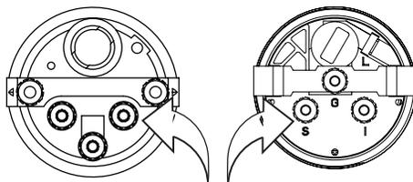
Electrical connections tighten 0.70 Nm max. (100 in. oz.)
