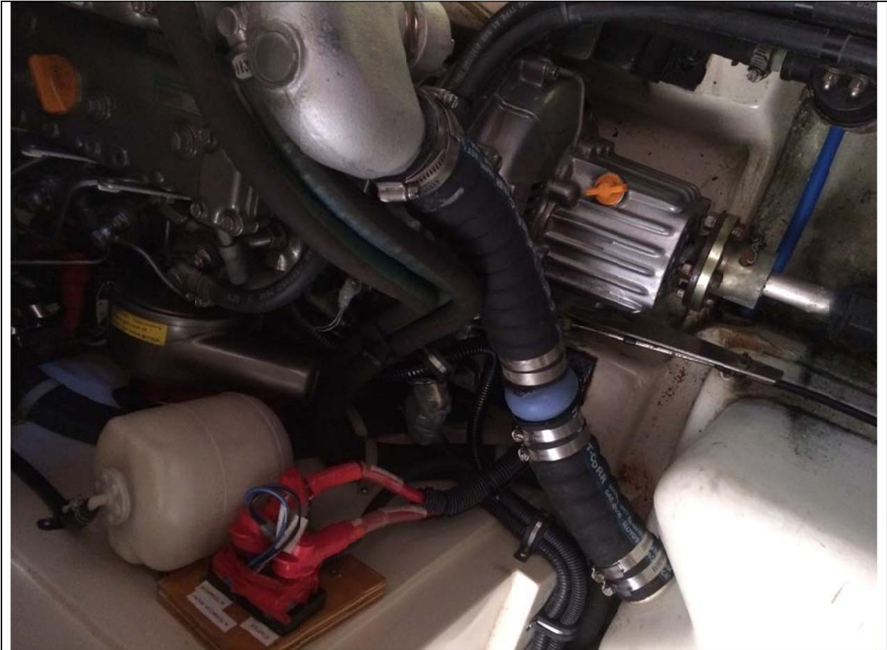
View From Top of Mixing Elbow. Used flexible hose 8" and 13" segments
